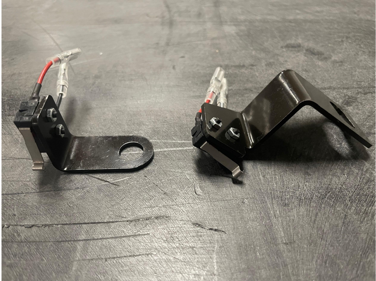
This is what the completed X-axis limit switch assembly should look like.
