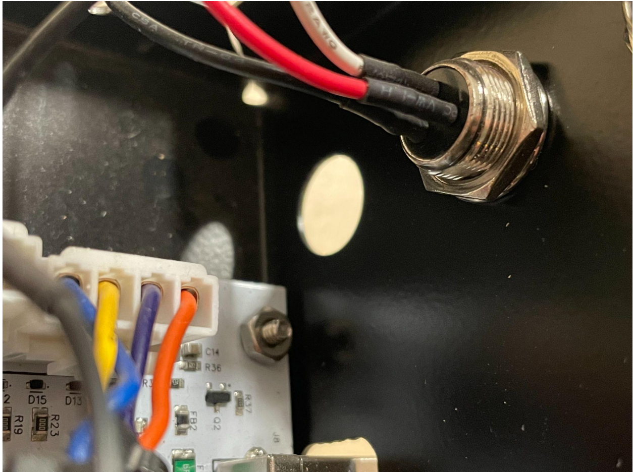
Identify the LIM port that was included with the limit switch kit. Note that its blade connectors are attached to wires that are color-coded yellow, green, and black.
