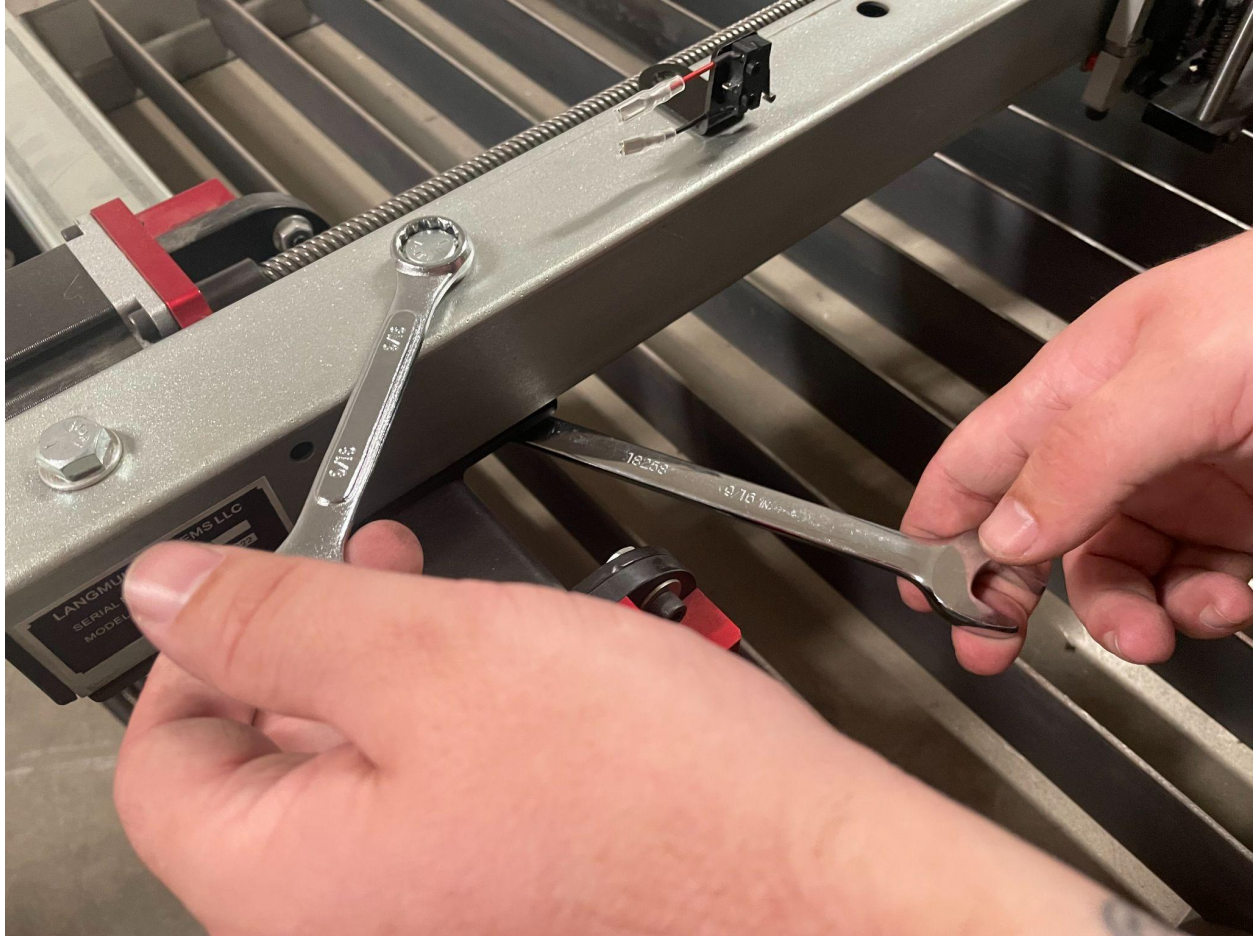
The X-axis limit switch bracket will mount in between the tube spacer and bolt pictured below.
