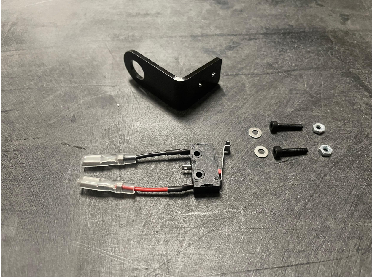
Identify the Y-axis limit switch mounting bracket, one of the limit switches, and the hardware that will mount the limit switch to the Y-axis bracket.
