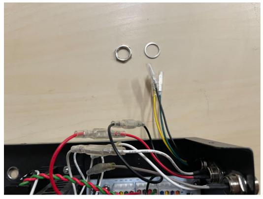
First, put the washer onto the blade connector wires. Then, put the ring nut onto the blade connector wires.
