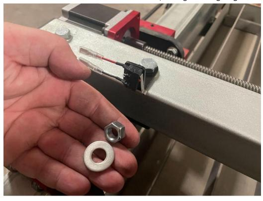
Ensure that the X-axis carriage interfaces with the limit switch before hitting the head of the bolt, as shown in the images below. Rotate the limit switch bracket around the bolt if necessary.
