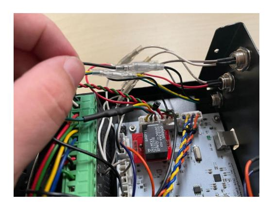
Your electronics enclosure is now ready to use limit switches, and can be installed back onto the leg tube of your CrossFire machine.
