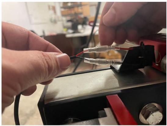
Connect the other end of the LIM cable to the LIM port that is installed in the EXP slot of the electronics enclosure.
