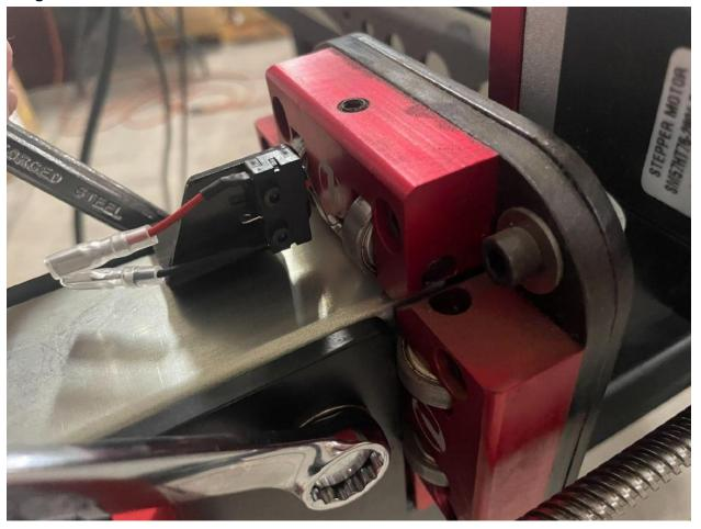
Your limit switches are now installed onto your machine, and are ready to be connected to the LIM port of your electronics enclosure using the LIM cable.
