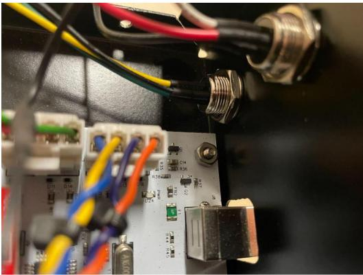
One the outside of the electronics enclosure, rotate the LIM port until it is in the desired position, then fully tighten the ring nut on the inside of the electronics enclosure to secure it in place.
