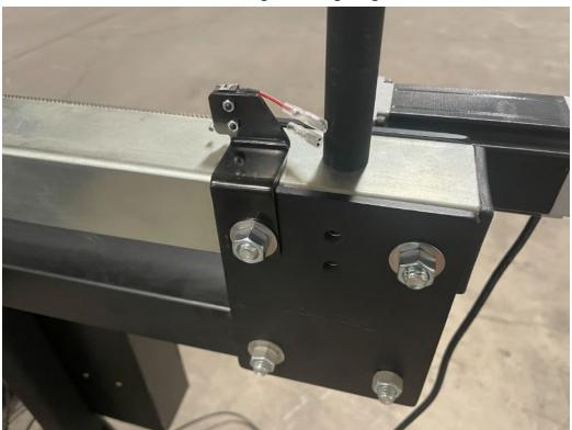
The Y-axis limit switch bracket has a significant amount of play compared to the X-axis limit switch mounting bracket installed in a previous step. Ensure that the bearing block of the Y-axis carriage interfaces with the switch before the bearings contact the stanchion plates.
