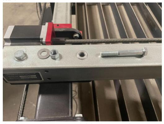
Line up the mounting hole of the X-axis limit switch bracket with the hole of the tube spacer, then pass the bolt through the set of holes.
