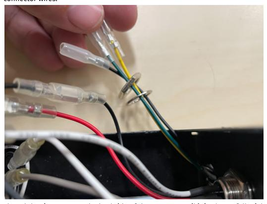
Thread the ring nut onto the backside of the LIM port until it is almost fully tightened.
