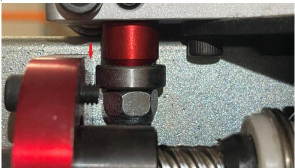
The same process is utilized to find the Y-axis soft limit. For **both the CrossFire and CrossFire PRO**, get the bearings of the Y-axis carriage as close to the stanchion plates as possible.
