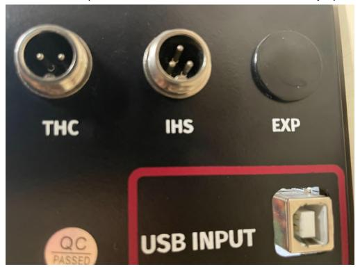
Inside of the electronics enclosure, squeeze the teeth of the plastic stopper blocking the EXP port slot.
