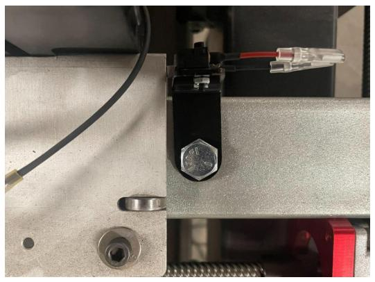
Once you are satisfied with the position of the X-axis limit switch, tighten the bolt and nut using two 9/16" box wrenches.
