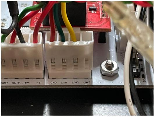
The black wiring harness will connect to the unused motion control board pins in the bottom left corner of the motion control board.
