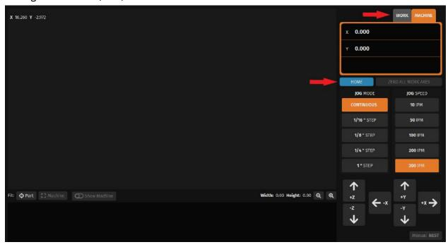
After the machine is homed, the DRO should read 0.000 for both X & Y. We'll be using the machine coordinate read-out to find the appropriate soft limits to set for your machine.
