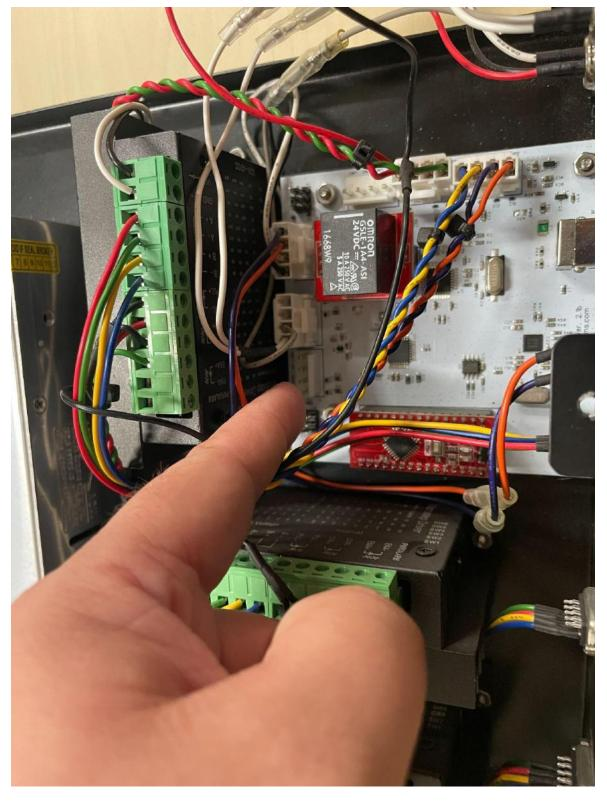
Connect the wiring harness in such a way that the motion control board position labeled 5v lines up to the black wire as shown. Firmly seat the connector into the mating connector on the board until it clicks in place.
