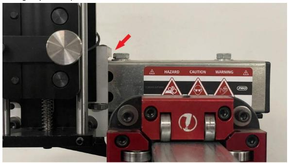
**For the CrossFire**, get the X-axis Carriage Assembly as close to the X-axis Bearing Mount as possible:
