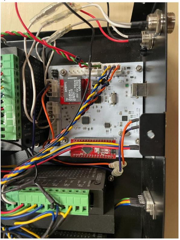
The green, yellow, and red wiring harness will connect to the unused motion control board pins in the top left corner of the motion control board.
