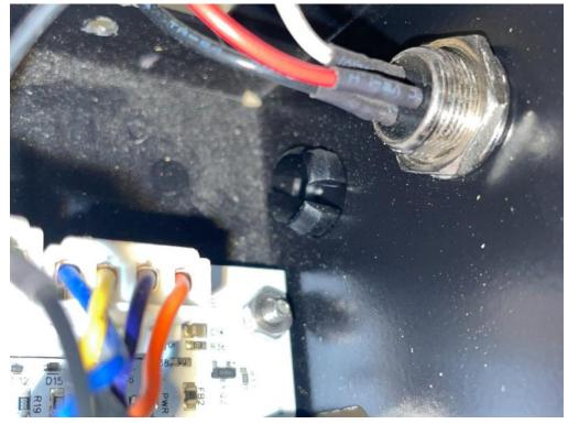
The plastic stopper should pop out of its position easily, allowing space to install the LIM port included with the limit switch kit into the EXP slot.
