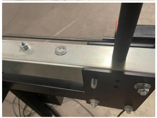
Pass the Y-axis limit switch bracket onto the bolt.
