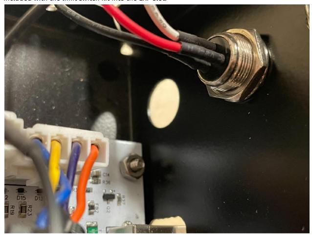
Identify the LIM port that was included with the limit switch kit. Note that its blade connectors are attached to wires that are color-coded yellow, green, and black.
