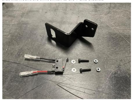
Orient the limit switches as shown below, and pass the bolts through the mounting holes on each switch. The washers will go in between the limit switches and the mounting brackets.
