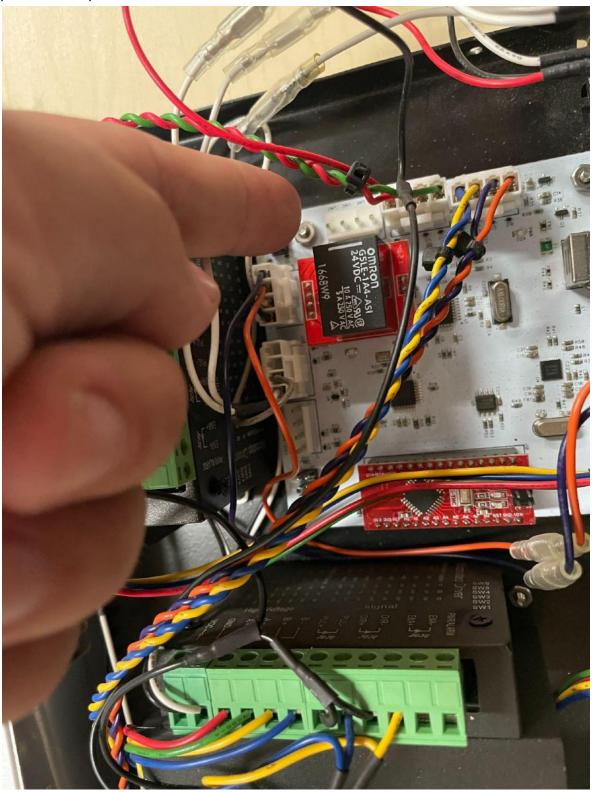
Connect the wiring harness in such a way that the motion control board position labeled GND lines up to the red wire, LIM1 lines up to the green wire, and LIM2 lines up to the yellow wire. Push the connector in firmly to click it into the mating board connector.
