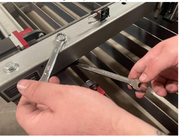
The X-axis limit switch bracket will mount in between the tube spacer and bolt pictured below.
