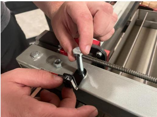
Your X-axis limit switch assembly should be oriented like this.
