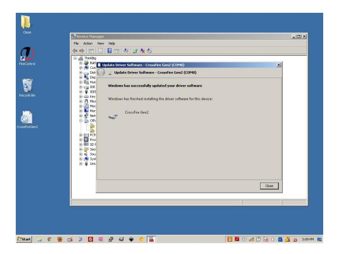
14.) You can now open FireControl and your device should Auto-connect appropriately. If it does not, click the drop down menu in machine connections and select the CrossFire machine. You may need to unplug and plug your USB cable back in for this to work after installing the drivers.
